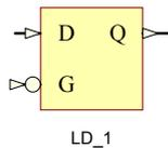
LD\_1 is a 1-bit transparent data latch with inverted gate.
