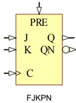
FJKPN is a single J-K-type flip-flop with J, K, and asynchronous preset (PRE) inputs and inverted (QN) and non-inverted (Q) outputs. When High, the asynchronous preset (PRE) input overrides all other inputs and sets the outputs Q to High and QN to Low. When PRE is Low, the Q and QN outputs respond to the state of the J and K inputs, as shown in the following truth table, during the Low-to-High clock transition.
