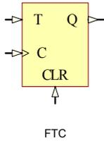
FTC is a synchronous, resettable toggle flip-flop. When High, the asynchronous clear (CLR) input overrides all other inputs and resets the data output (Q) Low. The Q output toggles, or changes state, when the toggle enable (T) input is High and CLR is Low during the Low-to-High clock transition.
