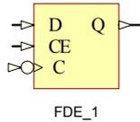
FDE\_1 is a D-type negative edge flip-flop with clock enable (CE).
