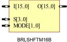
When MODE input is set to “11”, data from (I) input slice is shifted to the right (O) output slice controlled by select (S) inputs. The trailing output (O) slice is filled with 1.
