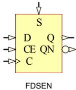
FDSSEN is a D-type positive edge flip-flop with clock enable (CE) and synchronous set (S) and inverted (QN) and non-inverted (Q) outputs.
