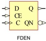
FDEN is D-type flip-flop with clock enable and inverted and non-Inverted outputs.
