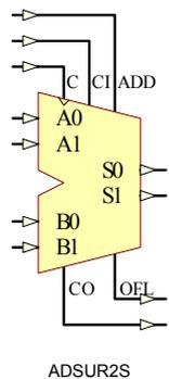
example, if component ADSUR4 is used to add 8 (1000) and 9 (1001) together, the resulting sum will be 17 (1 0001), which is out of the 4-bit unsigned binary range, thus CO will be 1. Again, CO is active High in add mode and active Low in subtract mode. Also OFL is ignored in unsigned binary operations.
