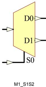
Mn\_B1B2, Mn\_S1S2, M1\_S1B2 are various  $n$ -bit data width 1-to-2 demultiplexers, available in bus-to-bus, pin-to-pin and pin-to-bus versions.
