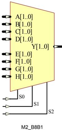
Mn\_B8B1, Mn\_S8S1, M1\_B8S1, Mn\_B8B1\_SB, Mn\_S8S1\_SB and M1\_B8S1\_SB are various  $n$ -bit data width 8-to-1 multiplexers, available in bus-to-bus, pin-to-pin and bus-to-pin versions.
