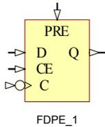
FDPE\_1 is a D type negative edge flip-flop with clock enable (CE) and asynchronous preset (PRE).
