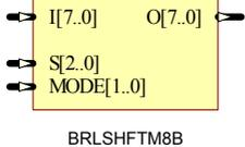
When MODE input is set to “10”, data from (I) input slice is shifted to the right (O) output slice controlled by select (S) inputs. The trailing output (O) slice is filled with 0.
