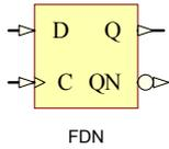
FDN is a D-type positive edge trigger flip-flop with inverted (QN) and non-inverted (Q) output. Input data (D) is loaded into the non inverted (Q) and inverted (QN) outputs during the Low-to-High clock (C) transition.
