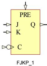
FJKP\_1 is a single J-K-type negative-edge triggered flip-flop with J, K, and asynchronous preset (PRE) inputs and data output (Q). When High, the asynchronous preset (PRE) input overrides all other inputs and sets the Q output High. When PRE is Low, the Q output responds to the state of the J and K inputs, as shown in the following truth table, during the High-to-Low clock transition.
