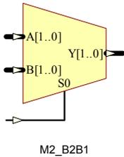
Mn\_B2B1, Mn\_S2S1, M1\_B2S1 are various  $n$ -bit data width 2-to-1 multiplexers, available in bus-to-bus, pin-to-pin and bus-to-pin versions.
