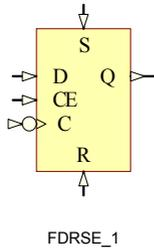
FDRSE\_1 is a D-type negative edge flip-flop with synchronous reset (R), set (S) and clock enable (CE). They are available in 1, 2, 4 or 8 bit bus or single pin versions.
