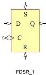
FDSR\_1 is a D-type negative edge flip-flop with synchronous set (S) and reset (R).
