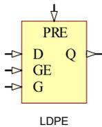
LDPE is a 1-bit transparent data latch with asynchronous preset and gate enable.
