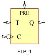
FTP\_1 is a negative-edge toggle flip-flop with toggle enable and asynchronous preset. When the asynchronous preset (PRE) input is High, all other inputs are ignored and output Q is set High. When toggle-enable input (T) is High and PRE is Low, output Q toggles, or changes state, during the High-to-Low clock (C) transition.
