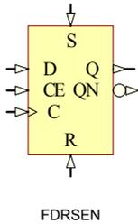
FDRSEN is a D-type positive edge flip-flop with synchronous reset (R), set (S) and clock enable (CE) and inverted (QN) and non-inverted (Q) outputs. They are available in 1, 2, 4 or 8 bit bus or single pin versions.
