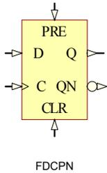
FDCPN is a D type positive edge flip-flop with asynchronous preset (PRE) and clear (CLR) and inverted (QN) and non-inverted (Q) outputs.
