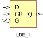
LDE\_1 is a 1-bit transparent data latch with gate enable and inverted gate.
