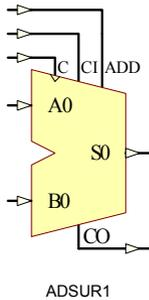
ADSUR1 is a 1-Bit cascadable registered full adder/subtractor. It adds or subtracts two input bits (A0, B0) with a carry-in (CI) during the Low-to-High clock (C) transition, producing a result (S0) and a carry-out (CO).
