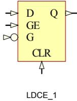
LDCE\_1 is a 1-bit Transparent Data Latch with Asynchronous Clear, Gate Enable, and Inverted Gate.
