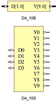
D4\_10 is an inverted one-hot decoder. It decodes valid BCD input logic ensuring that all outputs remain off for all invalid binary input conditions. The BCD logic is connected to inputs  $D[3..0]$ , with the resulting inverted one-hot decoded logic appearing on outputs  $Y[9..0]$ .
