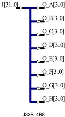
This component takes one *m*-bit input bus and maps to *p*, *n*-bit output buses. The following components are available:
