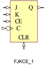
FJKCE\_1 is a single J-K-type negative-edge triggered flip-flop with J, K, clock enable (CE), and asynchronous clear (CLR) inputs and data output (Q). When High, the asynchronous clear (CLR) overrides all other inputs and resets the Q output Low. When CLR is Low and CE is High, Q responds to the state of the J and K inputs, as shown in the following truth table, during the High-to-Low clock transition. When CE is Low, the clock transitions are ignored and the state of Q remains unchanged.
