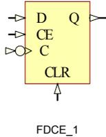
FDCE\_1 is a D type negative edge flip-flop with clock enable (CE) and asynchronous clear (CLR). When clear (CLR) is High, all other inputs are ignored and output (Q) is set to Low. When clear (CLR) is Low and clock enable (CE) is High, input data (D) is loaded into the output (Q) on the High-to-Low clock (C) transition. When clock enable (CE) is Low and clear (CLR) is Low, clock transitions are ignored and output (Q) does not change state.
