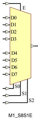
*Mn\_B8B1E*, *Mn\_S8S1E*, *M1\_B8S1E*, *Mn\_B8B1E\_SB*, *Mn\_S8S1E\_SB*, and *M1\_B8S1E\_SB* are various  $n$ -bit data width 8-to-1 multiplexers with enable, available in bus-to-bus, pin-to-pin and bus-to-pin versions.
