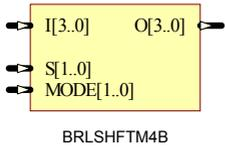
BRLSHFTM are 4, 8, 16 and 32 bit fill mode bi-directional barrel shifters. Direction and fill mode is chosen by using the shift mode (MODE) input.
