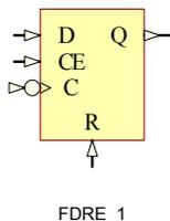
FDRE\_1 is a D-type negative edge flip-flop with clock enable (CE) and synchronous reset (R).
