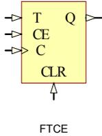
FTCE is a toggle flip-flop with toggle and clock enable and asynchronous clear. When the asynchronous clear (CLR) input is High all other inputs are ignored and the data output (Q) is reset Low. When CLR is Low and toggle enable (T) and clock enable (CE) are High, Q output toggles, or changes state, during the Low-to-High clock (C) transition. Clock transitions are ignored and the state of Q remains unchanged when CE is Low.
