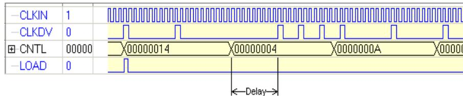
Expected output when Load is held Low and new CNTL input is loaded. A delay due to the internal counter can be expected between the next CLKDV output transitions.
