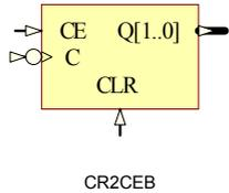
CR2CE, CR4CE, CR8CE, CR16CE, CR32CE are respectively 2-, 4-, 8-, 16-, 32-bit negative-edge binary ripple counters with clock enable and asynchronous clear.
