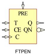
FTPEN is a toggle flip-flop with toggle and clock enable and asynchronous preset. When the asynchronous preset (PRE) input is High, all other inputs are ignored and output Q is set High whilst QN is set Low. When the toggle enable input (T) is High, clock enable (CE) is High, and PRE is Low, outputs Q and QN toggle, or changes state, during the Low-to-High clock transition. Clock transitions are ignored and the state of the outputs remains unchanged when CE is Low.
