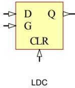
LDC is a 1-bit transparent data latch with asynchronous clear.
