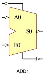
ADD1 is a 1-Bit full adder. The device adds two 1-bit words (A0, B0) and a carry-in (CI), producing a binary sum (S0) output and a carry-out (CO).
