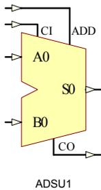
ADSU1 is a 1-Bit cascadable full adder/subtractor. It adds or subtracts two input bits (A0, B0) producing a result (S0) and a carry-out (CO).
