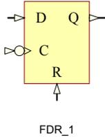
FDR\_1 is a D-type negative edge flip-flop with synchronous reset (R). They are available in 1, 2, 4 or 8 bit bus or single pin versions.
