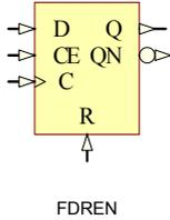
FDREN is a D-type positive edge flip-flop with clock enable (CE) and synchronous reset (R) and inverted (QN) and non-inverted (Q) outputs.
