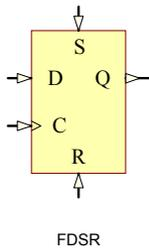
FDSR, FD2SR, FD4SR, FD8SR, FD16SR, FD32SR are, respectively 1-, 2-, 4-, 8-, 16-, 32-Bit D-type positive edge flip-flops with synchronous set (S) and reset (R).
