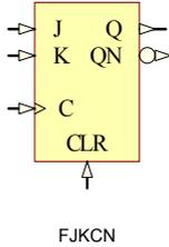
FJKCN is a single J-K-type flip-flop with J, K, and asynchronous clear (CLR) inputs and inverted (QN) and non-inverted (Q) outputs. When High, the asynchronous clear (CLR) input overrides all other inputs and resets the Q output Low and the QN output to High. When CLR is Low, the outputs respond to the state of the J and K inputs, as shown in the following truth table, during the Low-to-High clock (C) transition.
