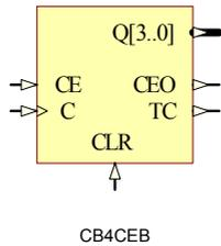
The Q outputs increment when clock enable (CE) is High during the Low-to-High clock transition. When CE is Low, clock transitions are ignored and outputs remain unchanged from the previous state.
