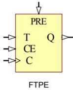
FTPE is a toggle flip-flop with toggle and clock enable and asynchronous preset. When the asynchronous preset (PRE) input is High, all other inputs are ignored and output Q is set High. When the toggle enable input (T) is High, clock enable (CE) is High, and PRE is Low, output Q toggles, or changes state, during the Low-to-High clock transition. Clock transitions are ignored and the state of Q remains unchanged when CE is Low.
