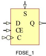
FDSE\_1 is a D-type negative edge flip-flop with clock enable (CE) and synchronous set (S).
