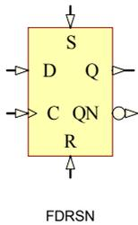
FDRSN is a D-type positive edge flip-flop with synchronous reset (R) and set (S) and inverted (QN) and non-inverted (Q) outputs.
