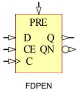
FDPEN is a D type positive edge flip-flop with clock enable (CE) and asynchronous preset (PRE).
