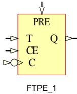
FTPE\_1 is a negative-edge toggle flip-flop with toggle and clock enable and asynchronous preset. When the asynchronous preset (PRE) input is High, all other inputs are ignored and output Q is set High. When the toggle enable input (T) is High, clock enable (CE) is High, and PRE is Low, output Q toggles, or changes state, during the High-to-Low clock transition. Clock transitions are ignored and the state of Q remains unchanged when CE is Low.
