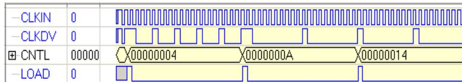
Expected output when Load is set to High and used to force the counter with new CNTL input.
