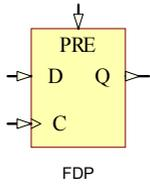
FDP, FD2P, FD4P, FD8P, FD16P, FD32P are, respectively 1-, 2-, 4-, 8-, 16-, 32-Bit D-type positive edge flip-flop with asynchronous preset (PRE). When preset (PRE) is High, all other inputs are ignored and output (Q) is set to High. When preset (PRE) is Low, Input data (D) is loaded into the output (Q) during Low-to-High clock (C) transition.
