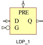
LDP\_1 is a 1-bit transparent latch with asynchronous preset.
