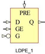
LDPE\_1 is a 1-bit transparent data latch with asynchronous preset and gate enable and inverted gate.
