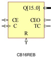
CB2RE, CB4RE, CB8RE, CB16RE, CB32RE are respectively 2-, 4-, 8-, 16-, 32-Bit Cascadable Binary Counters with Clock Enable and Synchronous Reset.
