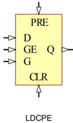
LDCPE is a 1-bit transparent data latch with asynchronous clear and preset and gate enable.
