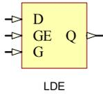
LDE is a 1-bit transparent data latch with gate enable.
