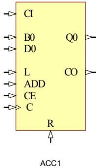
ACC1 is a 1-Bit cascadable loadable accumulator. It can add or subtract data to or from the contents of a 1-bit data register and store the result back into the register. The register can be loaded with a 1-bit word.
