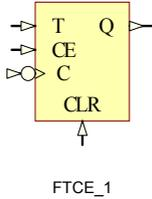
FTCE\_1 is a negative-edge toggle flip-flop with toggle, clock enable and asynchronous clear. When the asynchronous clear (CLR) input is High all other inputs are ignored and the data output (Q) is reset Low. When CLR is Low and toggle enable (T) and clock enable (CE) are High, Q output toggles, or changes state, during the High-to-Low clock (C) transition. Clock transitions are ignored and the state of Q remains unchanged when CE is Low.
