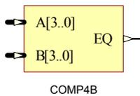
COMP2, COMP3, COMP4, COMP5, COMP6, COMP7, COMP8, COMP9, COMP10, COMP12, COMP16 and COMP32 are, respectively, 2-, 3-, 4-, 5-, 6-, 7-, 8-, 9-, 10-, 12-, 16- and 32-bit identity comparators. The equal output (EQ) of the identity comparator is High when the two words  $A_n - A_0$  and  $B_n - B_0$  are equal. When any two of the corresponding bits from each word are not the same, the EQ output is Low.
