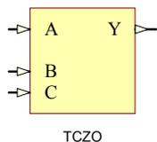
TCZO can output a true signal of A (A), a complement of A ( $\bar{A}$ ), a zero ('0') or a one ('1') to Y depending on the state of B and C.
