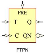
FTPN is a toggle flip-flop with toggle enable and asynchronous preset. When the asynchronous preset (PRE) input is High, all other inputs are ignored and output Q is set High whilst QN is set Low. When toggle-enable input (T) is High and PRE is Low, outputs Q and QN both toggle, or changes state, during the Low-to-High clock (C) transition.
