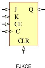
FJKCE is a single J-K-type flip-flop with J, K, clock enable (CE), and asynchronous clear (CLR) inputs and data output (Q). When High, the asynchronous clear (CLR) overrides all other inputs and resets the Q output Low. When CLR is Low and CE is High, Q responds to the state of the J and K inputs, as shown in the following truth table, during the Low-to-High clock transition. When CE is Low, the clock transitions are ignored and the state of Q remains unchanged.
