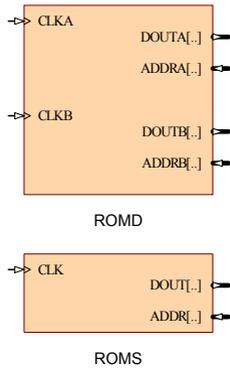
ROMS and ROMD are single and dual port read only memory. Data output (DOUT) is always active on the defined clock trigger and valid address (ADDR) input.
