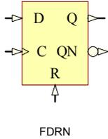
FDRN is a D-type positive edge flip-flop with synchronous reset (R) and inverted (QN) and non-inverted (Q) outputs.
