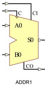
ADDR1 is a 1-Bit registered full adder. The device adds two 1-bit words (A0, B0) and a carry-in (CI) on the rising-edge of the clock input (C), producing a binary sum (S0) output and a carry-out (CO).
