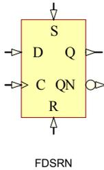
FDSRN is a D-type positive edge flip-flop with synchronous set (S) and reset (R) and inverted and non-inverted outputs.
