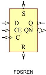
FDSREN is a D-type positive edge flip-flop with synchronous set (S), reset (R) and clock enable (CE) with inverted (QN) and non-inverted (Q) outputs.
