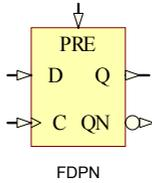
FDPN is a D-type positive edge flip-flop with asynchronous preset (PRE) and inverted (QN) and non-inverted (Q) outputs. They are available in 1, 2, 4 or 8 bit bus or single pin versions.
