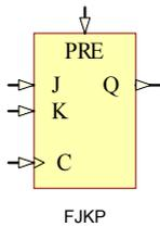
FJKP is a single J-K-type flip-flop with J, K, and asynchronous preset (PRE) inputs and data output (Q). When High, the asynchronous preset (PRE) input overrides all other inputs and sets the Q output High. When PRE is Low, the Q output responds to the state of the J and K inputs, as shown in the following truth table, during the Low-to-High clock transition.
