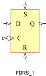
FDRS\_1 is a D-type negative edge flip-flop with synchronous reset (R) and set (S).
