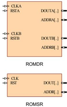
ROMSR and ROMDR are single and dual port read only memory with reset. When reset (RST) is High, data output (DOUT) is cleared on the defined clock trigger. When reset (RST) is Low, data output (DOUT) is always active on the defined clock trigger and valid address (ADDR) input.
