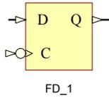
FD\_1 is a D-type negative edge trigger flip-flop. Input data (D) is loaded into the output (Q) during High-to-Low clock (C) transition.
