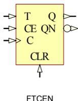
FTCEN is a toggle flip-flop with toggle and clock enable and asynchronous clear. When the asynchronous clear (CLR) input is High all other inputs are ignored and the data outputs Q is reset Low and QN is reset High. When CLR is Low and toggle enable (T) and clock enable (CE) are High, Q and QN outputs both toggle, or change state, during the Low-to-High clock (C) transition. Clock transitions are ignored and the state of the outputs remains unchanged when CE is Low.
