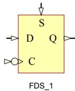
FDS\_1 is a D-type negative edge flip-flop with synchronous set (S).
