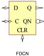
FDCN is a D type positive edge flip-flop with asynchronous clear (CLR) and inverted (QN) and non-inverted (Q) outputs. When clear (CLR) is High, all other inputs are ignored and inverted (QN) and non-inverted (Q) outputs are set to High and Low respectively. Input data (D) is loaded into the outputs when clear (CLR) is Low on the Low-to-High clock (C) transition.
