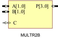
MULTR2, MULTR4, MULTR8, MULTR16, MULTR18, MULTR32 are respectively 2x2, 4x4, 8x8, 16x16, 18x18, 32x32 registered signed multipliers. They perform multiplication of two signed values from the two inputs (A and B) on the rising-edge of the clock input (C) and produce a product (P).
