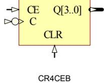
The counter increments when clock enable input (CE) is High during the High-to-Low clock transition. When CE is Low, clock transitions are ignored and the outputs remain in the same state as the previous clock cycle.
