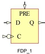
FDP\_1 is a D-type negative edge flip-flop with asynchronous preset (PRE).
