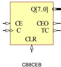
Larger counters can be created by connecting the CEO output of the first stage to the CE input of the next stage and connecting C and CLR inputs in parallel. When cascading counters, use the CEO output if the counter uses the CE input; use the TC output if it does not.
