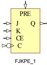
FJKPE\_1 is a single J-K-type negative-edge triggered flip-flop with J, K, clock enable (CE), and asynchronous preset (PRE) inputs and data output (Q). When High, the asynchronous preset (PRE) overrides all other inputs and sets the Q output High. When PRE is Low and CE is High, the Q output responds to the state of the J and K inputs, as shown in the truth table, during the High-to-Low clock (C) transition. Clock transitions are ignored and the state of Q remains unchanged when CE is Low.
