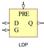
LDP is a 1-bit transparent latch with asynchronous preset.
