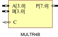
Input A and B are 2-, 4-, 8-, 16-, 18, 32-Bit length and output P is 4-, 8-, 16-, 32-, 36, 64-Bit length for MULTR2, MULTR4, MULTR8, MULTR16, MULTR18, MULTR32 respectively. All input and output values are represented in two's-complement format.
