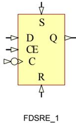
FDSRE\_1 is a D-type negative edge flip-flop with synchronous set (S) and reset (R) and clock enable (CE).
