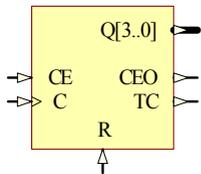
CD4RE is a cascadable binary-coded-decimal (BCD) counter with clock enable and synchronous reset.
