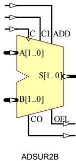
ADSUR2, ADSUR4, ADSUR8, ADSUR16 and ADD32 are, respectively 2-, 4-, 8-, 16 and 32-Bit cascadable registered full adders and full subtractors with signed (two's-complement) and unsigned binary operations.
