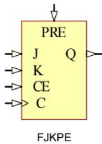
FJKPE is a single J-K-type flip-flop with J, K, clock enable (CE), and asynchronous preset (PRE) inputs and data output (Q). When High, the asynchronous preset (PRE) overrides all other inputs and sets the Q output High. When PRE is Low and CE is High, the Q output responds to the state of the J and K inputs, as shown in the truth table, during the Low-to-High clock (C) transition. Clock transitions are ignored and the state of Q remains unchanged when CE is Low.
