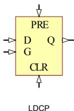
LDCP is a 1-bit transparent data latch with asynchronous clear and preset.
