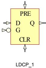
LDCP\_1 is a 1-bit transparent data latch with asynchronous clear and preset and inverted gate.
