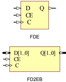
FDES, FD2E, FD4E, FD8E, FD16E and FD32E are, respectively 1-, 2-, 4-, 8-, 16-, 32-Bit D-type positive edge flip-flops with clock enable (CE).
