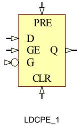
LDCPE\_1 is a 1-bit transparent data latch with asynchronous clear and preset and inverted gate enable.
