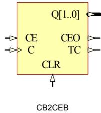
CB2CE, CB4CE, CB8CE, CB16CE and CB32CE are, respectively 2-, 4-, 8-, 16-, 32-Bit Cascadable Binary Counters with Clock Enable and Asynchronous Clear.
