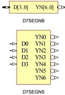
D7SEGN decodes a 4-bit binary-coded-decimal (BCD) input for 7-Segment Common-Anode LED Display. Outputs of D7SEGN are Active Low.
