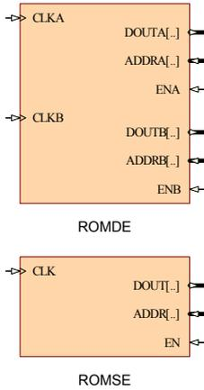
ROMSE and ROMDE are single and dual port read only memory with enable. When enable (EN) is High, data transfer is disabled and no change occurs at data output (DOUT). When enable (EN) is Low, data output (DOUT) is always active on the defined clock trigger and valid address (ADDR) input.
