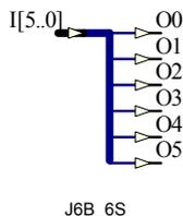
This component takes an *n*-bit input bus and maps each bit to *n* single output pins. The following components are available:
