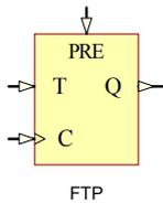
FTP is a toggle flip-flop with toggle enable and asynchronous preset. When the asynchronous preset (PRE) input is High, all other inputs are ignored and output Q is set High. When toggle-enable input (T) is High and PRE is Low, output Q toggles, or changes state, during the Low-to-High clock (C) transition.
