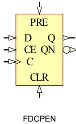
FDCPEN is a D type positive edge flip-flop with clock enable (CE) and asynchronous preset (PRE) and clear (CLR) and inverted (QN) and non-inverted (Q) outputs.
