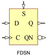
FDSN is a D-type positive edge flip-flop with synchronous set (S) and inverted (QN) and non-inverted (Q) outputs.
